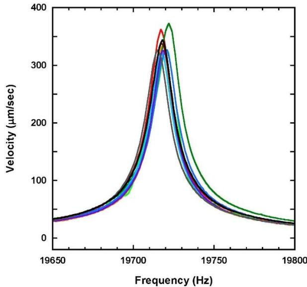
Figure 4. Long term stability of the vibration spectrum. Each curve shows a measurement taken at different times during one day.
