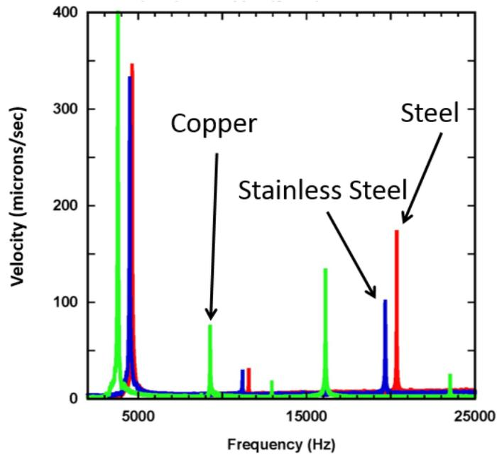
Figure 2. Measured vibration spectra for 6" cylinders of copper (green curve), steel (red), and stainless steel (blue).
