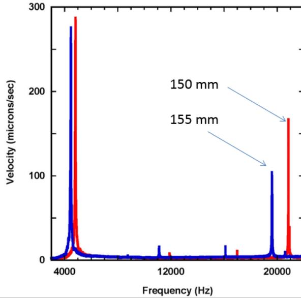
Figure 3. Measured vibration spectrum of cylinders of length 150 mm (red curve) and 155 mm (blue).
