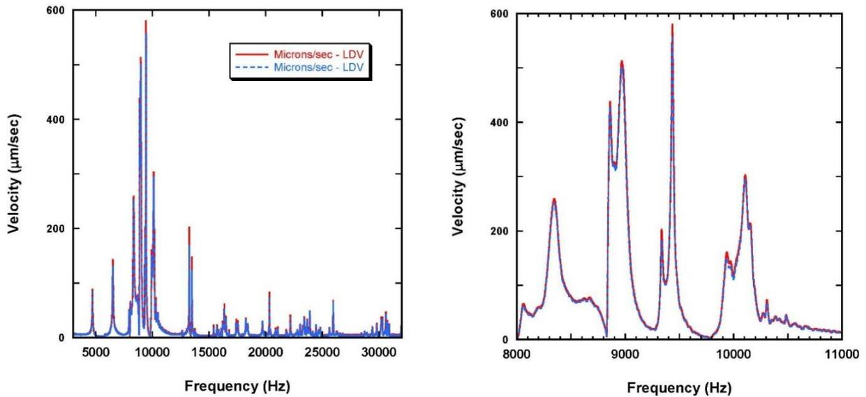
Figure 8. Vibrational Spectrum of a complex aluminum extrusion.
