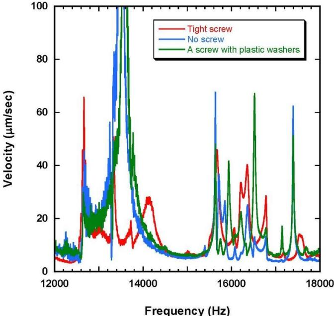
Figure 10. Acoustical spectrum of the extruded component with different changes.
