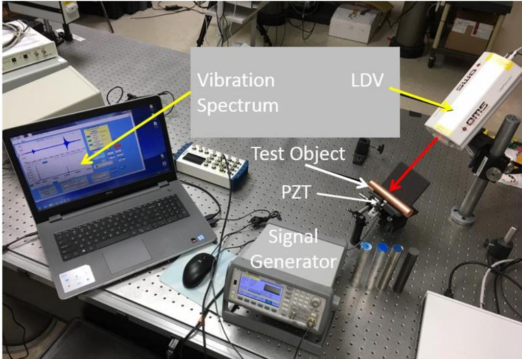
Figure 1. Experimental Setup for measuring the acoustical spectrum of a metal cylinder.
