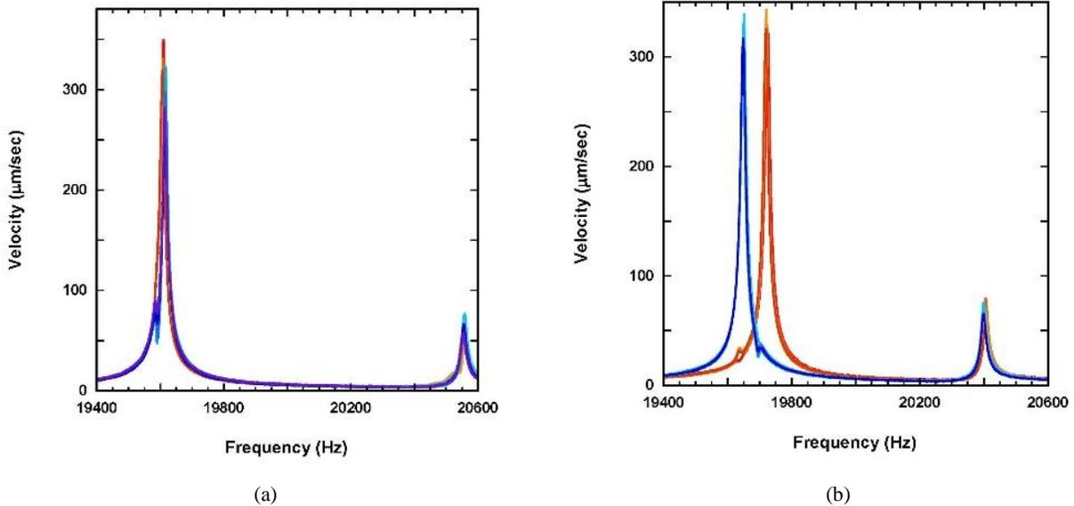
Figure 6. Comparing the spectrum of (a) unmodified with (b) modified cylinder. The red curve shows the spectrum when the excitation is parallel to the drilled hole, while the blue curve is when the excitation is perpendicular to the hole.
