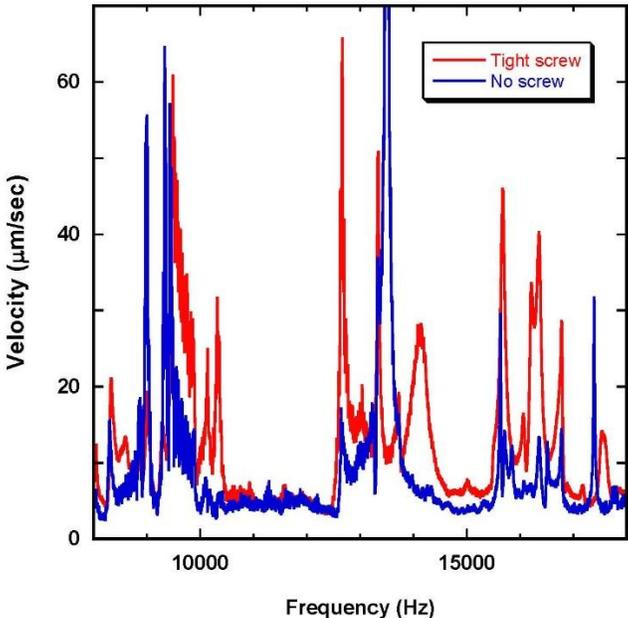
Figure 9. Acoustical spectrum for a T-Slotted extrusion with (red) and without a screw (blue) in the component.
